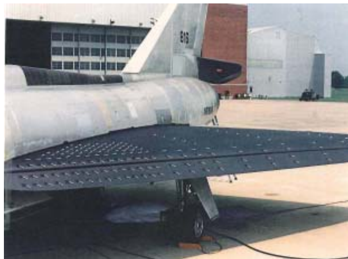
Figure 5 - The Leading Edge Flap installation on the NASA F-106B parked on the ramp at NASA Langley Research Center in 1988. Tufts have been installed to aid in flow pattern visualization.
