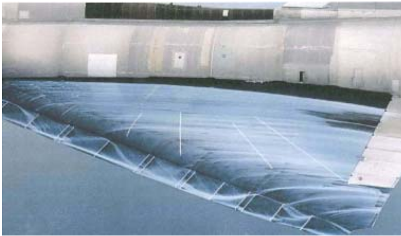
Figure 6 - Flow patterns etched in an oil film on the flap and upper wing surface after a flight indicate multiple vortices originated on the flap and swept back over the wing, unlike the single vortex lying neatly on the flap as predicted by the early flow models.
